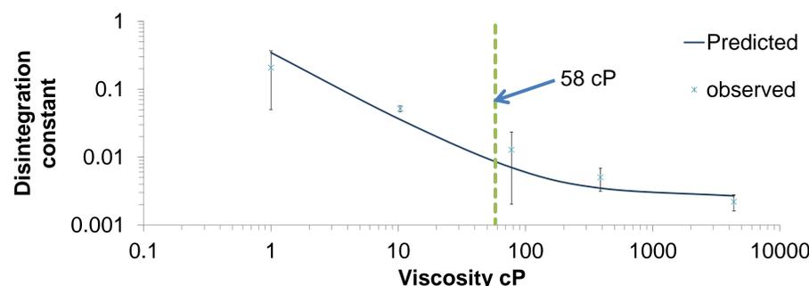
Figure 2: Relationship between viscosity and disintegration constant.
